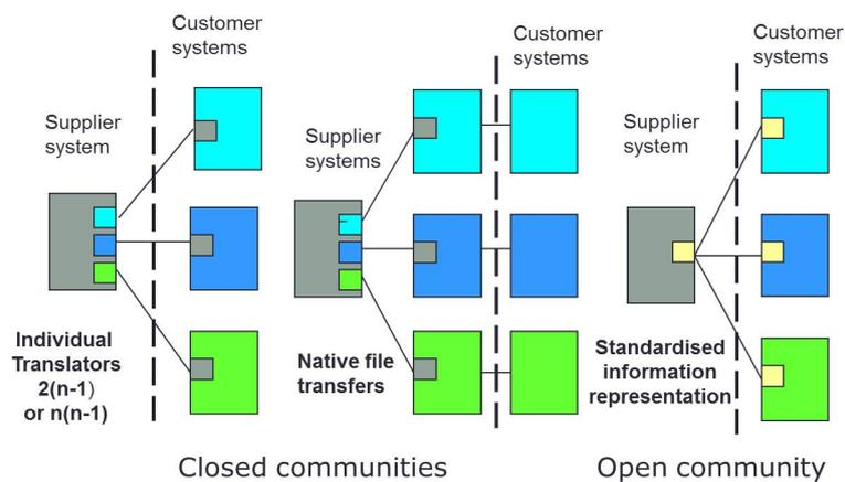
Figure 1 Strategies for the exchange of engineering product data between different systems in a supply chain.
