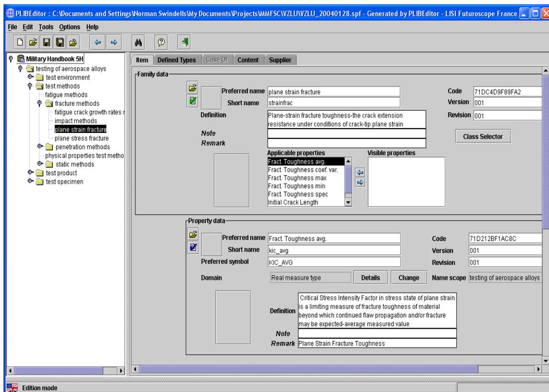
Figure 7 Screen shot of a portion of a dictionary of testing methods and their properties conforming to ISO 13584
