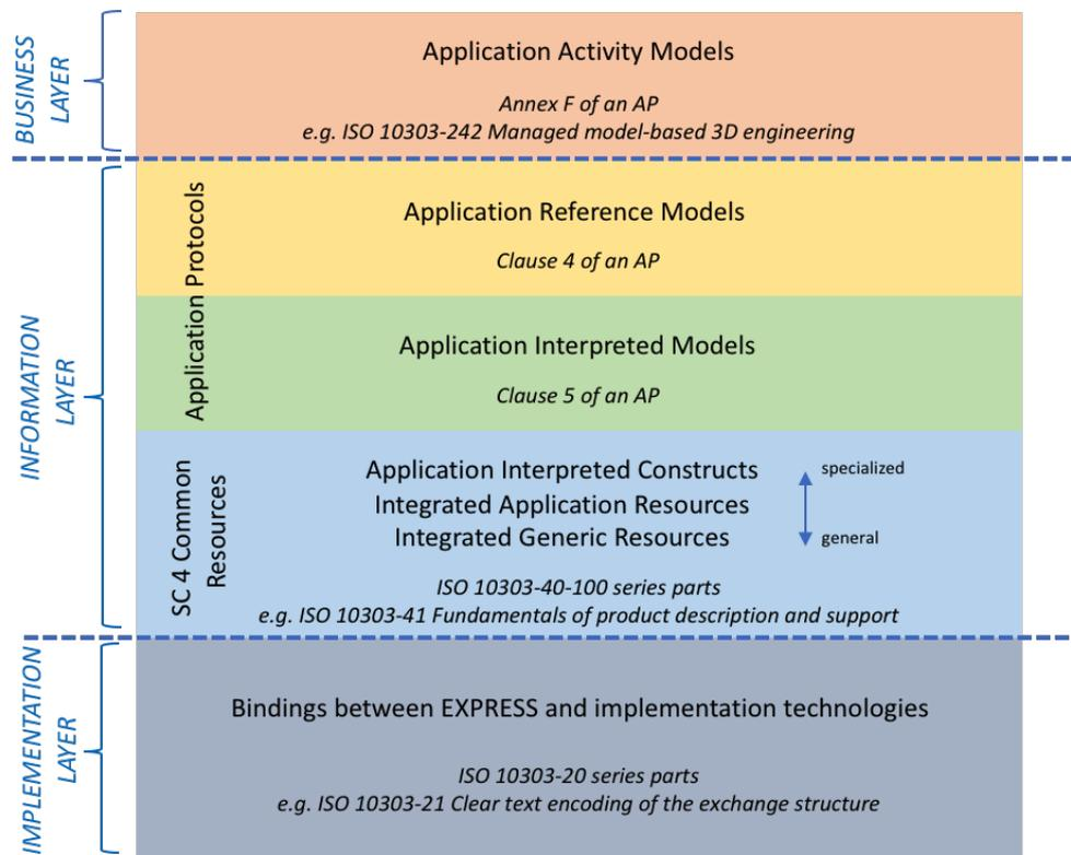
Figure 8. The fundamental architecture of a STEP standard document
