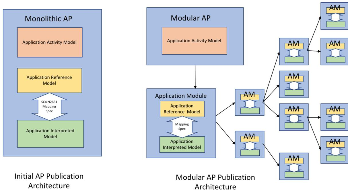
Figure 9 Comparison between the monolithic and modular architecture of a STEP standard document
