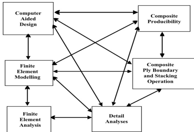
Figure 5 Interconnections between design, analysis and manufacturing information for composite material products
