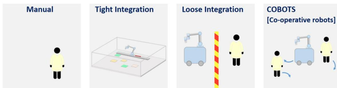
FIGURE 10: Four generic means to integrate automated unit operations into automated workflows.
