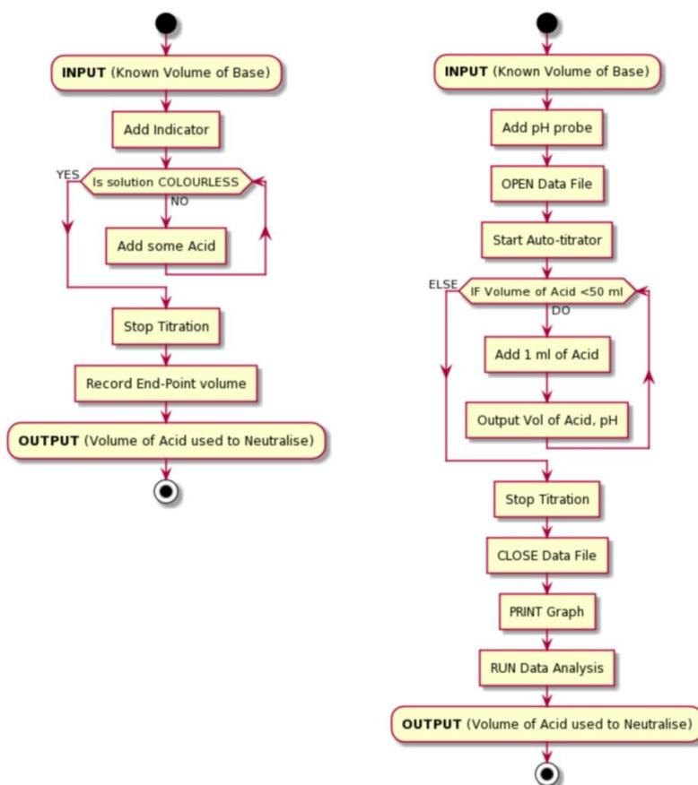
**FIGURE 6: The task list for a manual titration unit operation (left), and a comparable task list for a computer controlled titration (right).**
