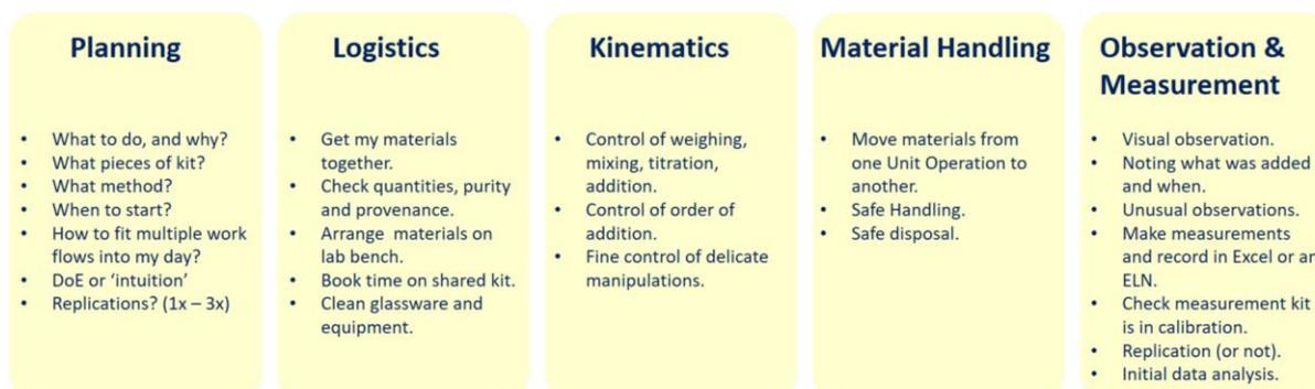
**FIGURE 9: The end-to-end process of lab work will involve planning, logistics, kinematics, handing, and observation steps. There is often little advantage in attempting to include all of these processes in an automation approach. More frequently a few key unit operations or joined up elements of the workflow will be automated to make a substantial improvement in the efficiency of the activity.**
