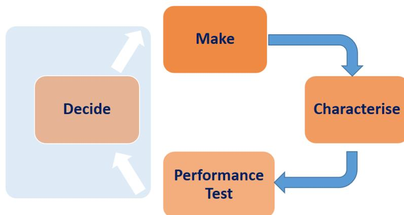
**FIGURE 5: Adding an algorithmic Decide step into an existing Make - Characterise - Performance test loop creates a 'closed-loop' that significantly speeds up the end-to-end process.**
