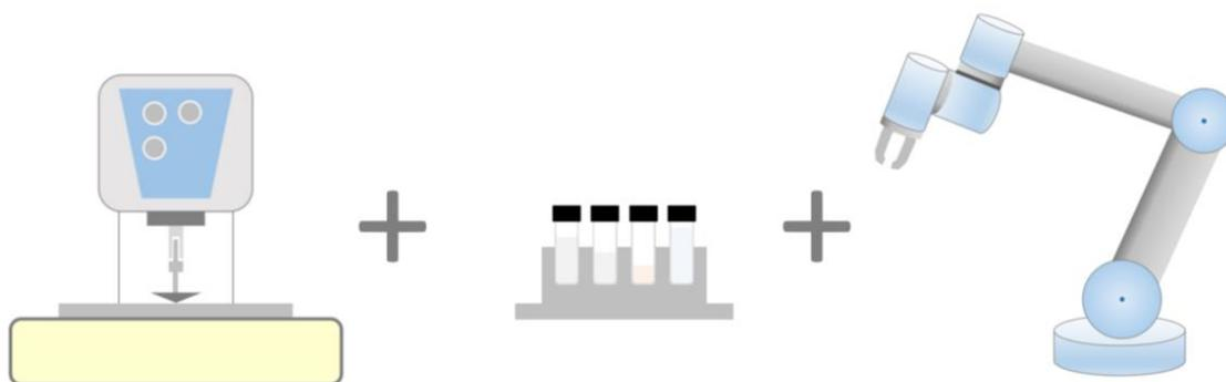
**FIGURE 7: A schematic example of how an existing rheometer, plus an off the shelf robotic arm, can be used to create an automated rheometer Unit Operation.**
