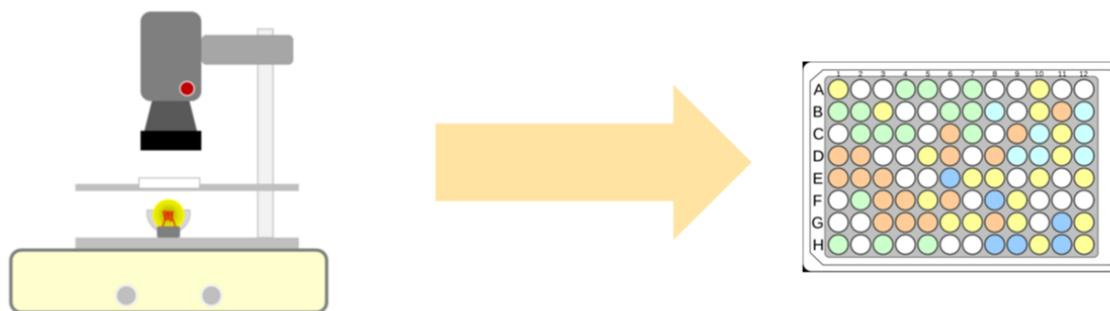
**FIGURE 8: A schematic example of how an existing serial measurement, made using a point imaging device such as a microscope, can be implemented in a 96 well plate format that can be scanned on e.g. a flatbed optical scanner.**
